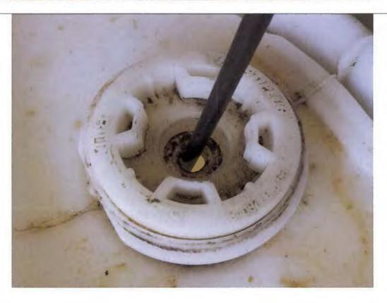
Photograph documenting the gap in the top of the Azone 15 sodium hypochlorite solution container between its cap and the chemical injection line.
