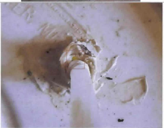
Photograph documenting the hole in the small hole in the top of the sodium hypochlorite solution container at Plant No. 2.
