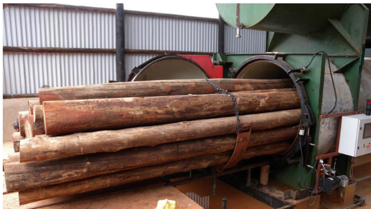
Figure 2. A mini-rail car with treated poles leaving the treatment cylinder.
