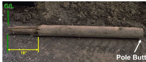
Figure 9. The section of a failed southern pine pole from the groundline and below.
