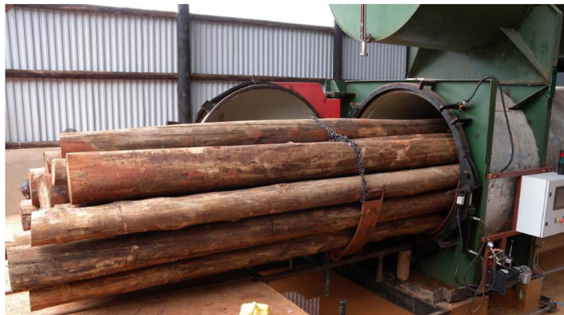
Figure 2. A mini-rail car with treated poles leaving the treatment cylinder.
