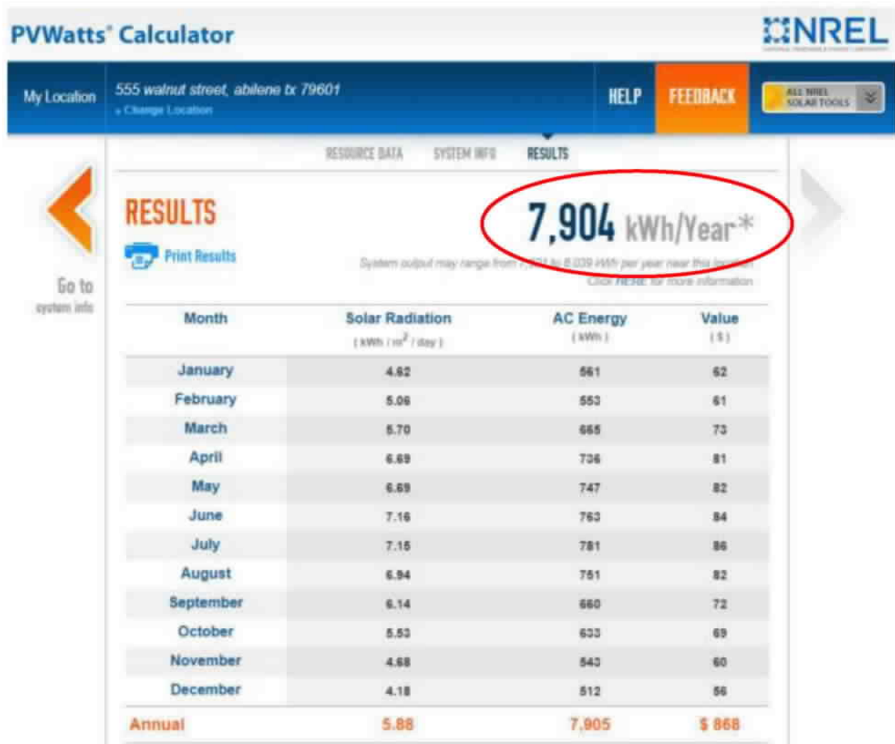
Figure 5. RES Solar PV—PVWatts Output Screen for Step 4
