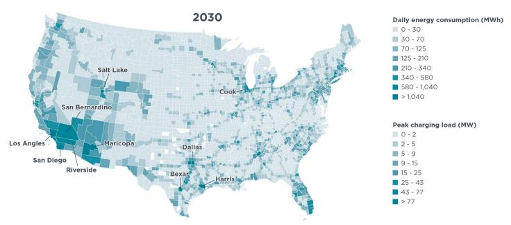
**Figure ES1.** County-level electric MHDV daily energy consumption in 2030 based on projections of near-term ZEV market growth (data labels indicate the ten counties with the highest energy consumption from electric MHDV).
