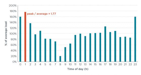
Figure 6. Typical fleet charging load profile for Class 4-8 MHDVs in California in 2030.
