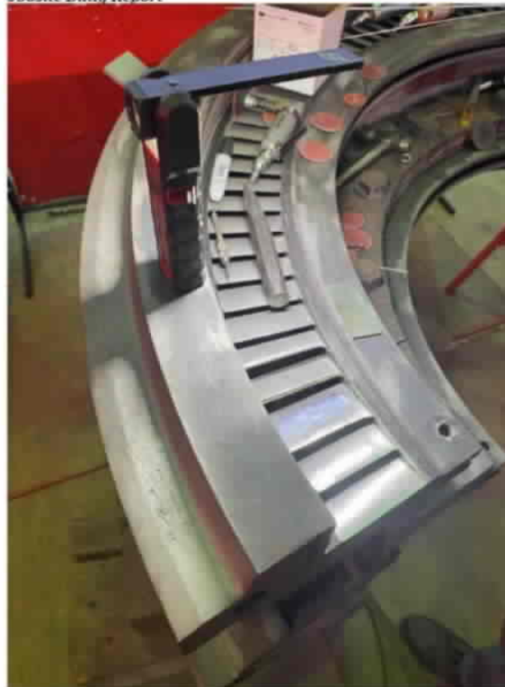
13 th Stage Stationary Blade Repair
