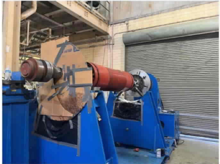
Generator Exciter Field on Lathe For Ring Machining
