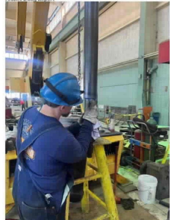
Lapping and Contact Checking on Re-heat Seal Valve Pressure Seats
