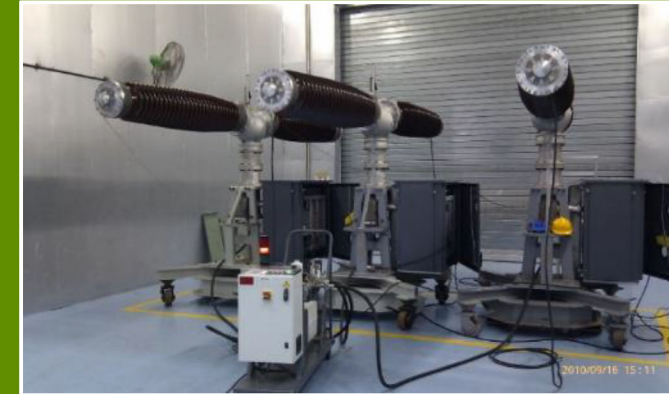
Live tank breaker assembly and testing complying with latest quality and EHS standards
