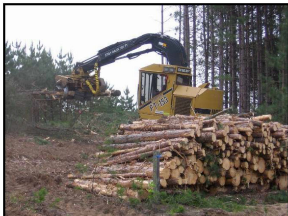
Figure 9 Whole Tree Processor Clearing
