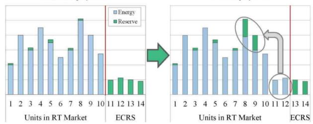
The illustration shows that when units 11 and 12 start and produce energy, other units ramp down to keep supply and demand in balance. In this case, it is units 8 and 9 that ramp down and provide spinning reserves to the system. Stated differently, offline 10-minute reserves were exchanged for online 10-minute spinning reserves when ECRS was deployed.
