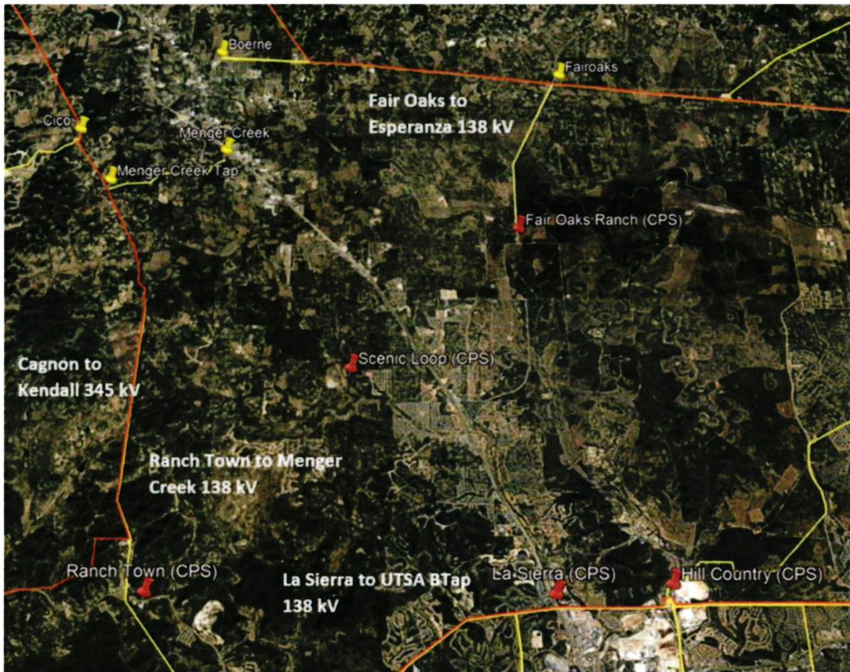
Figure 16 Transmission lines in the area surrounding the proposed Scenic Loop Substation
