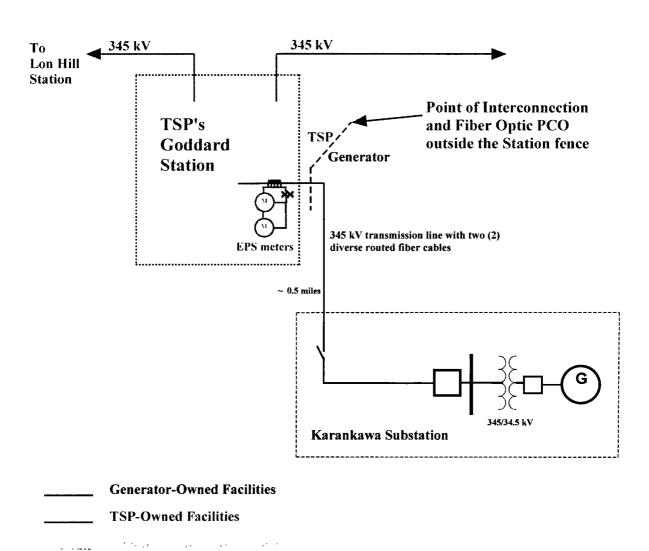
Conceptual One-Line Drawing of Point of Interconnection
