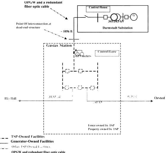
OPGW and redundant fiber optic cable
