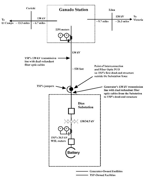
Conceptual One-Line Drawing of Point of Interconnection
