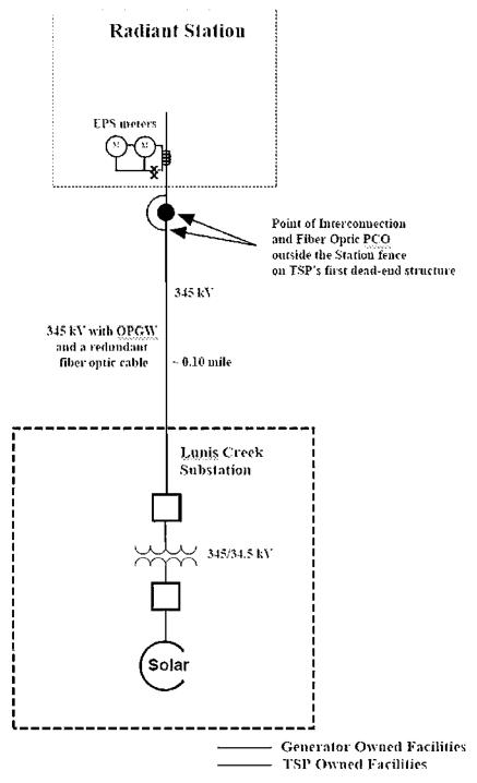
Distances as shown are conceptual and not to scale; Station and Substation not shown completely.
