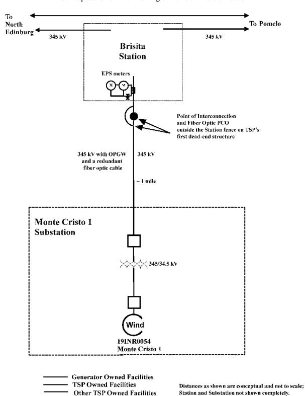
Conceptual One-Line Drawing of Point of Interconnection
