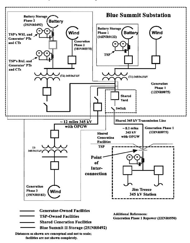
Conceptual One-Line Drawing of Point of Interconnection:
