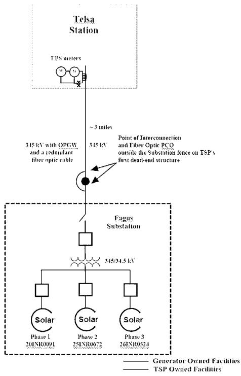
Distances as shown are conceptual and not to scale; Station and Substation not shown completely.
