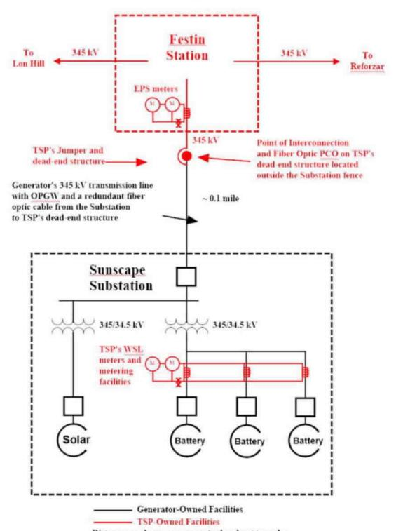
Distances as shown are conceptual and not to scale; Station, Substation and lines are not shown completely.
