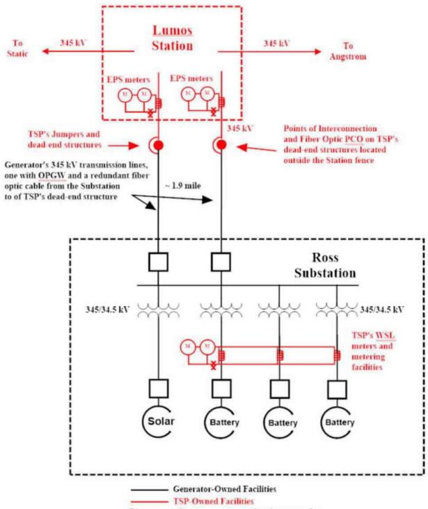
Distances as shown are conceptual and not to scale; Station, Substation and lines are not shown completely.
