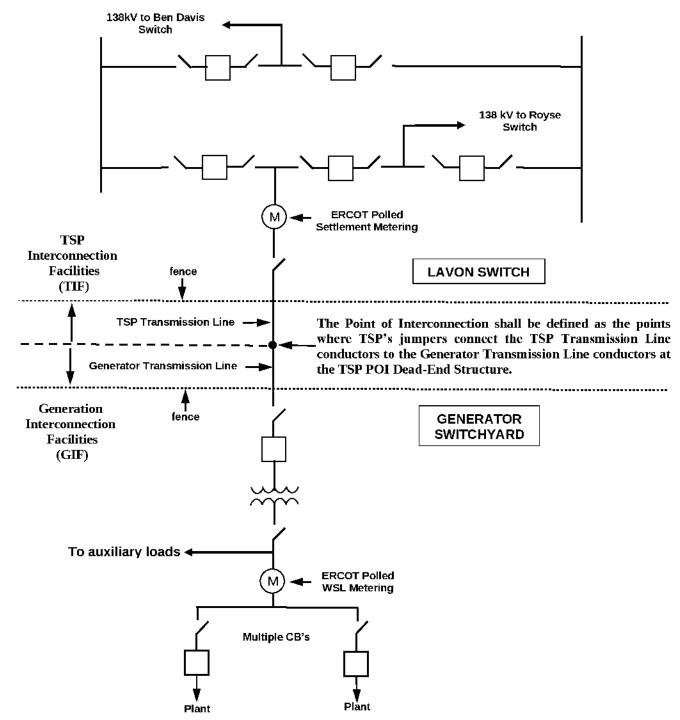
Note 1: This simplified one-line diagram is for illustration only and shall not be used for purposes of design, construction or operations.
