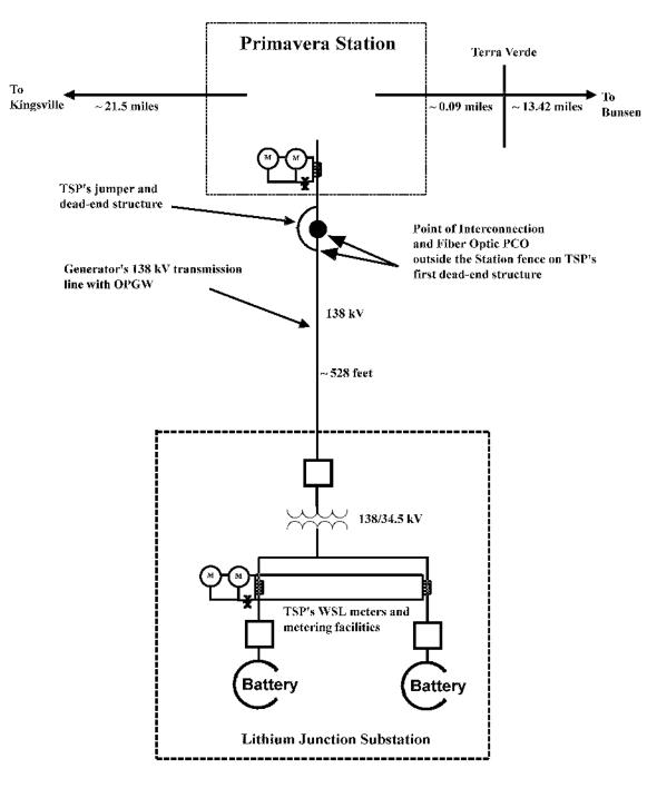
Conceptual One-Line Drawing of Point of Interconnection
