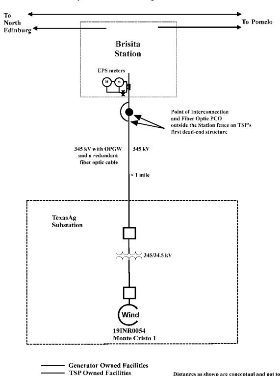
Conceptual One-Line Drawing of Point of Interconnection
