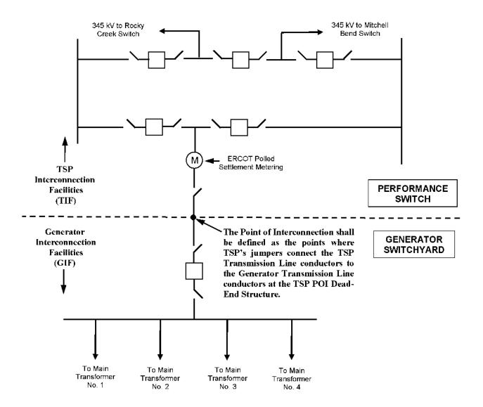
Note: This simplified one-line diagram is for illustration only and shall not be used for purposes of design, construction or operations.
