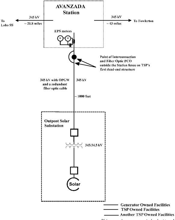
Conceptual One-Line Drawing of Point of Interconnection
