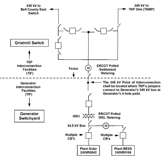
Note: This simplified one-line diagram is for illustration only and shall not be used for purposes of design, construction or operations.
