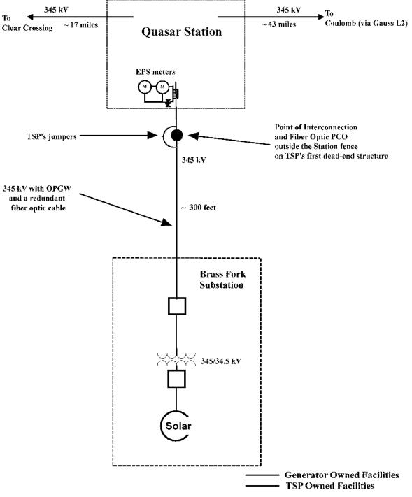
Conceptual One-Line Drawing of Point of Interconnection
