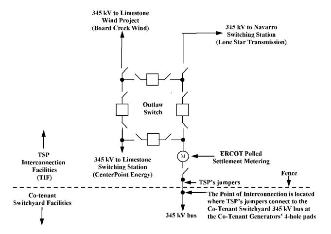
Note: This one-line diagram is for illustration only and shall not be used for purposes of design, construction or operations.
