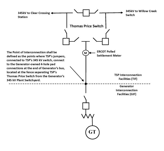
**<u>NOTE</u>**: This one-line diagram is for illustration only and shall not be used for purposes of design construction or operations.
