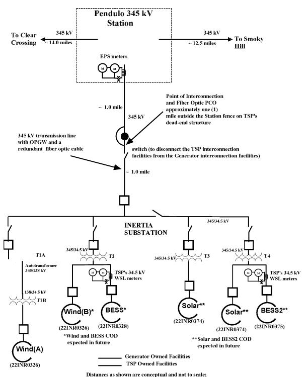
Station and Substation not shown completely.
