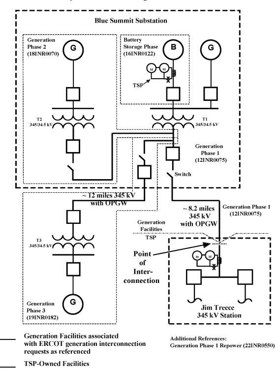
Conceptual One-Line Drawing of Point of Interconnection
