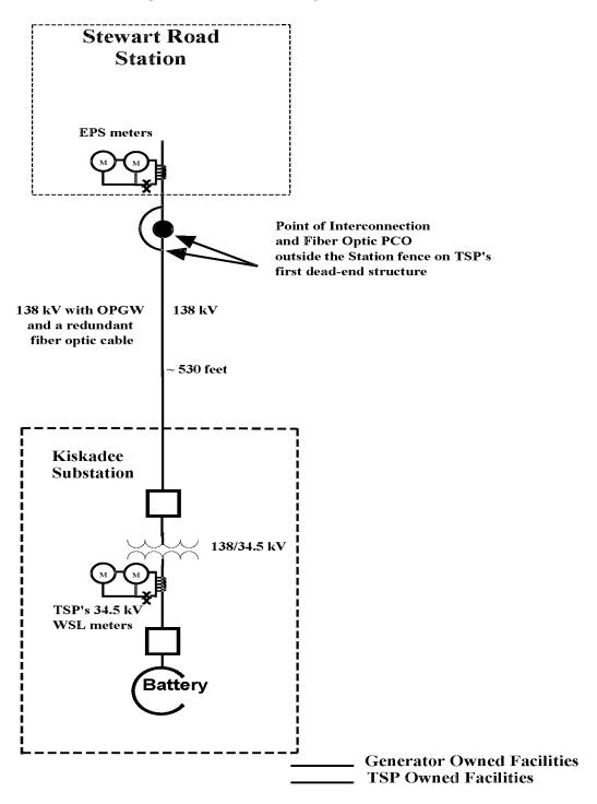
Distances as shown are conceptual and not to scale; Station and Substation not shown completely.
