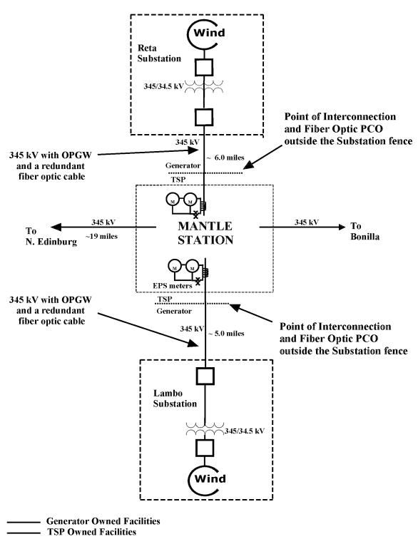
Conceptual One-Line Drawing of Point of Interconnection
