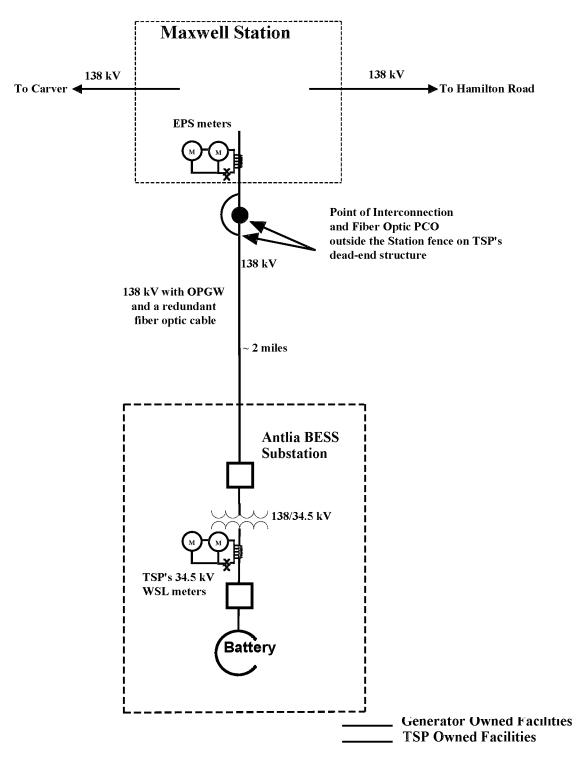
Distances as shown are conceptual and not to scale; Station and Substation not shown completely.
