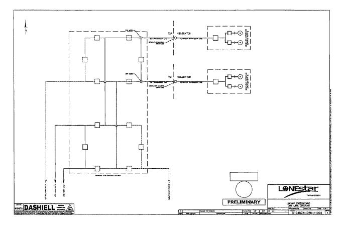
Attachment C-2 Conceptual One-Line Drawing of Point of Interconnection
