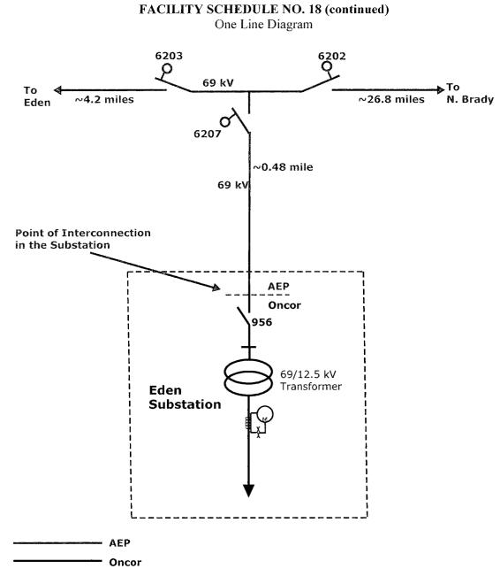
Distances as shown are conceptual and not to scale; Substation not shown completely.
