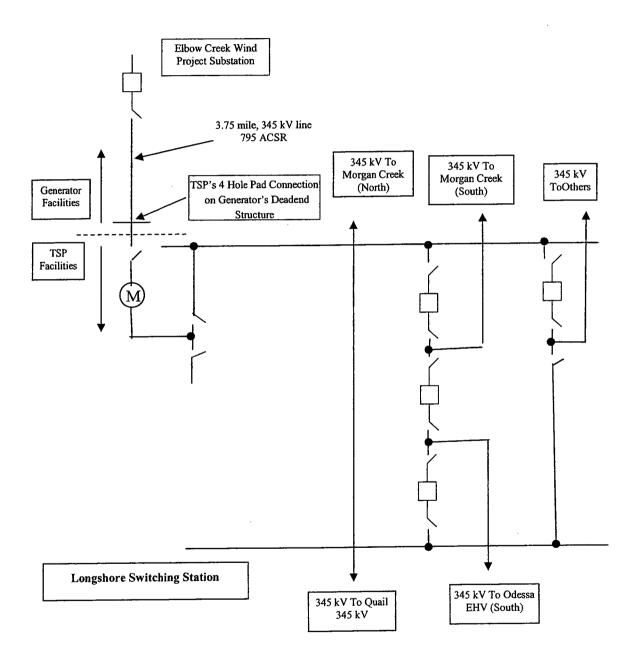
Note: This one-line diagram is for illustration only and shall not be used for purposes of design, construction or operations
