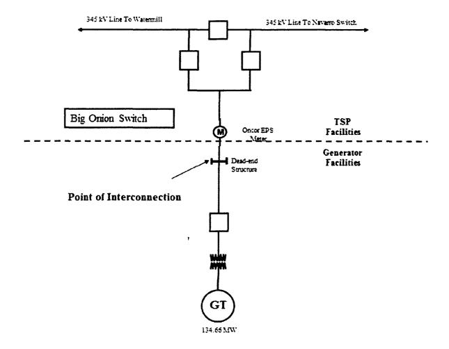
NOTE: This one-line diagram is for illustration only and shall not be used for purposes of design construction or operations.
