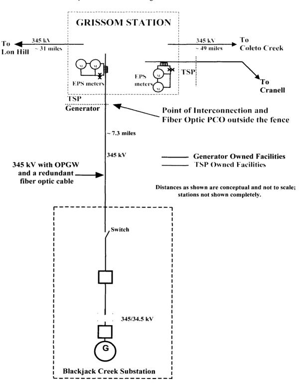
Conceptual One-Line Drawing of Point of Interconnection
