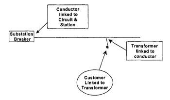
The diagram above provides a simple visual picture of the data that has to be linked together in order to identify an individual customer to a particular circuit. Where key linkage information is not readily available, an expensive field inventory has to be made to collect the necessary data to provide the customer connectivity links.
